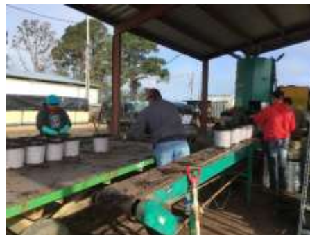
Figure 2. Automated Pot Fillers
